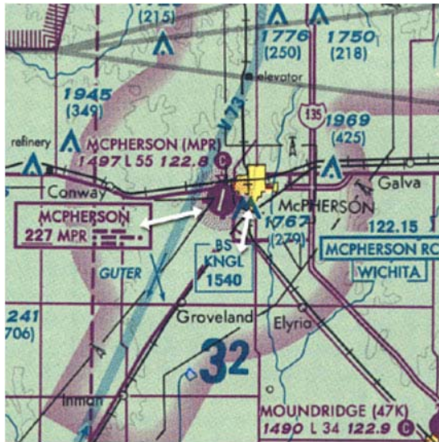
Figure 1: McPherson airport has an NDB, shown by the dotted circle around the airport. A commercial broadcast station, KNGL, is also located near the airport.
